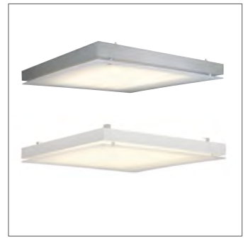
T5 GRILL UNI Wall and ceiling light, T16, square, white or silver-grey with frosted acrylic glass, 4xG5 T16, 4x24W (excl.), incl. electronic ballast. L/W/H: 60.5/60.5/8.5 cm EEL=A 1)
