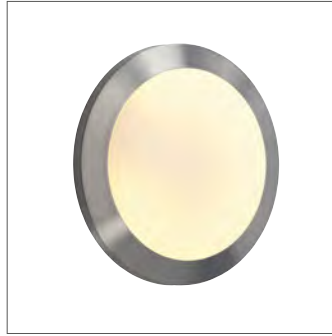
CL 135 T16 R Wall and ceiling light, round, white plastic/aluminium, T5 T16-R, energy saving light, 40W (excl.), incl. electronic ballast. Ø/H: 45/10.5 cm EEL=A 1)
